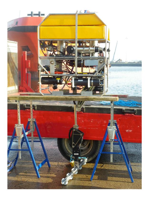
The above picture shows the full reach of a customised Hydro-Lek 5 function manipulator holding a simulated fuel rod – the manipulator can be retracted fully within the ROV frame.
